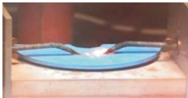
Fig.1. Flashover on silicone rubber specimen
