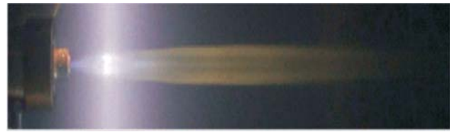
Fig. 4. Argon. Supersonic nozzle: d'' = 0, 215 mm; D = 3, 80 mm;
